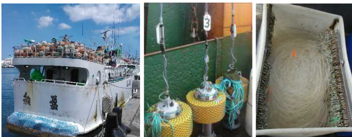
Figure 3.3: Photographs showing marker buoys (left), radio buoys (centre) and monofilament branch lines (right) (Source: CapMarine, 2015).
