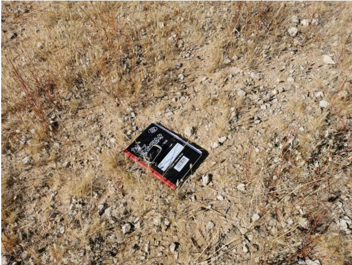
Figure 11: Typical soils (sandy gravel and calcrete) observed within the project site area
