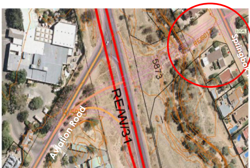
Figure 5: Erven 6018 and 6019 will have a new road passing due to the new link between Aviation Road and Springbok
