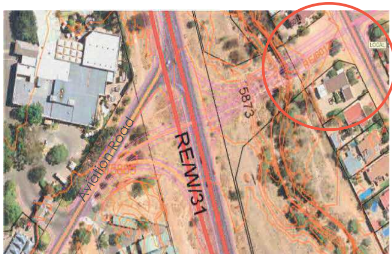
Figure 3: Erven 6018 and 6019 will have a new road passing due to the new link between Aviation Road and Springbok Street.
