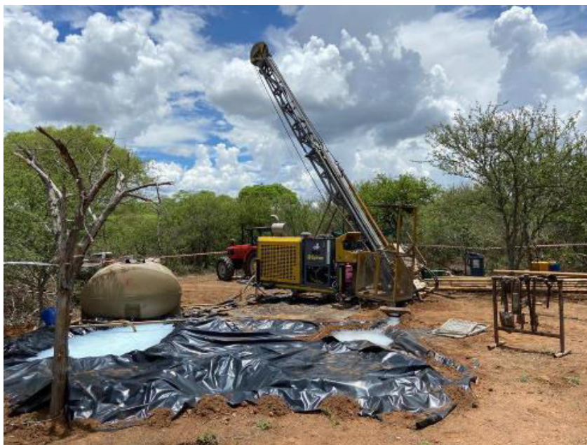
Figure 22 - Drill rig and sumps at site: NANAND000024
