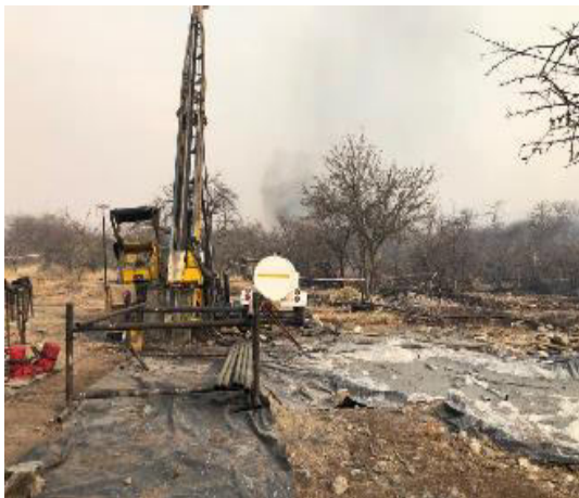
Figure 16 - Drill rig and sumps at site: NANAND000021
