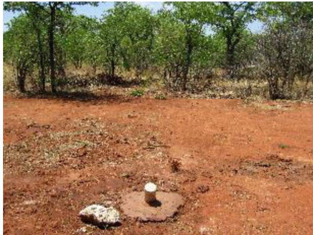
Post drilling - cleaned drill-site
