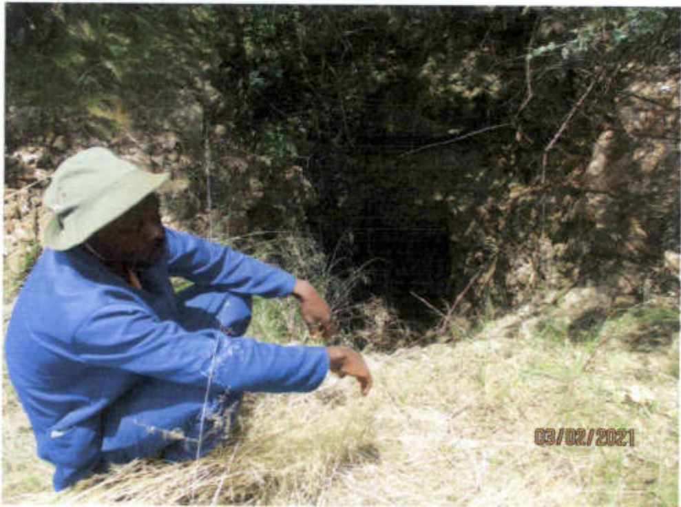
PHOTO 1: Shows the entrance to an old prospecting shaft put down in the 1960's on the northern extension of the orebody that was worked 1981-1887. The shaft, sunk on the orebody, carries the brecciated gossanous vein in the left and right hand walls of the inclined shaft. This has been sampled.
