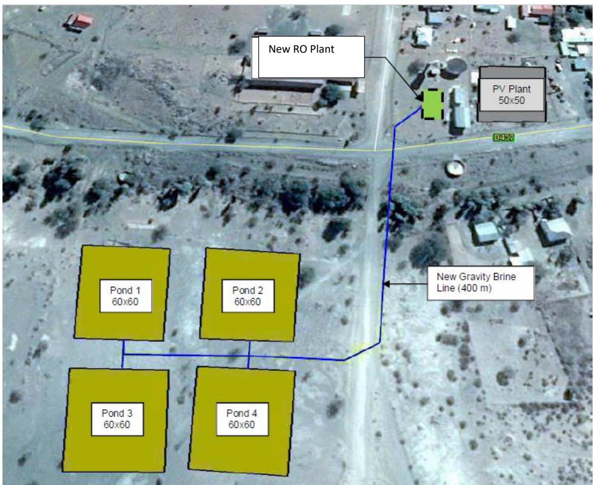
Figure 4: New Infrastructure Added to the Bethanie Plant
