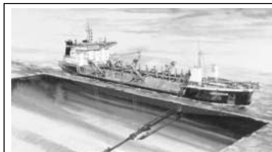
Photo 6-2 An example of a trailing suction hopper dredger (from Vlasblom, 2003)
