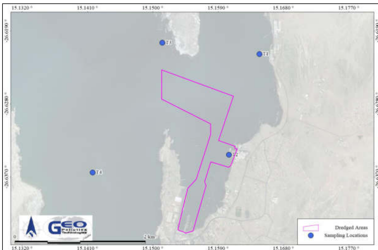
Figure 9-10 Locations for determining baseline turbidity conditions during the 2015 dredging exercise (Botha and Faul, 2015)
