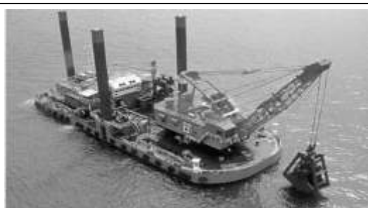
Photo 6-1 Typical grab dredger (from Vlasblom, 2003)
