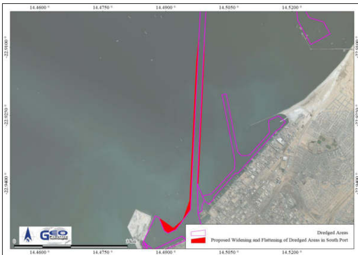
Figure 6-3 Widening and flattening of the entrance channel and manoeuvring areas of the South Port
