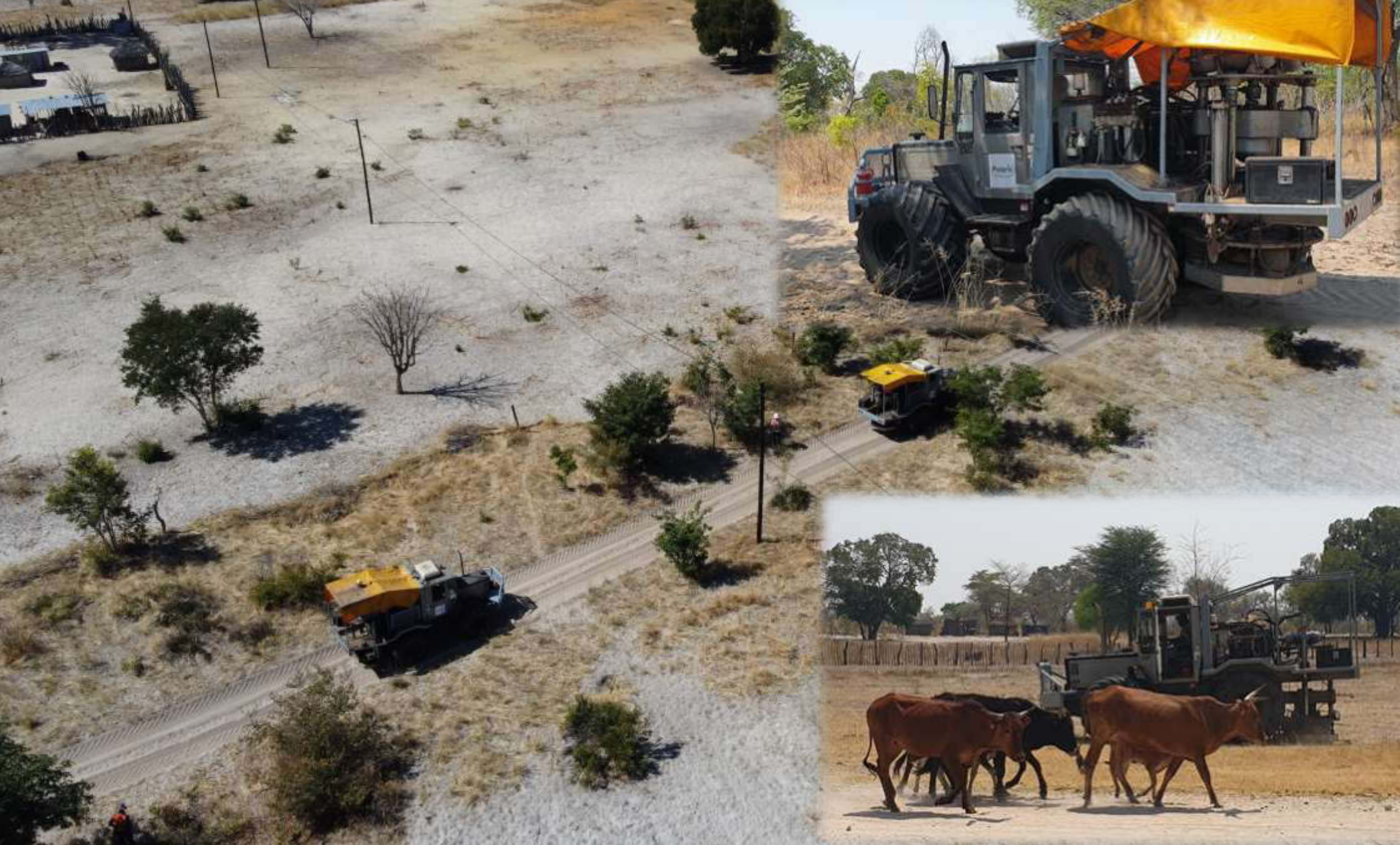
Plate 3.1: The Explorer 860 being used for the Phase I 2D seismic survey along Line 6 (main photo) and lines 9 and 4 top and bottom inserts respectively.
