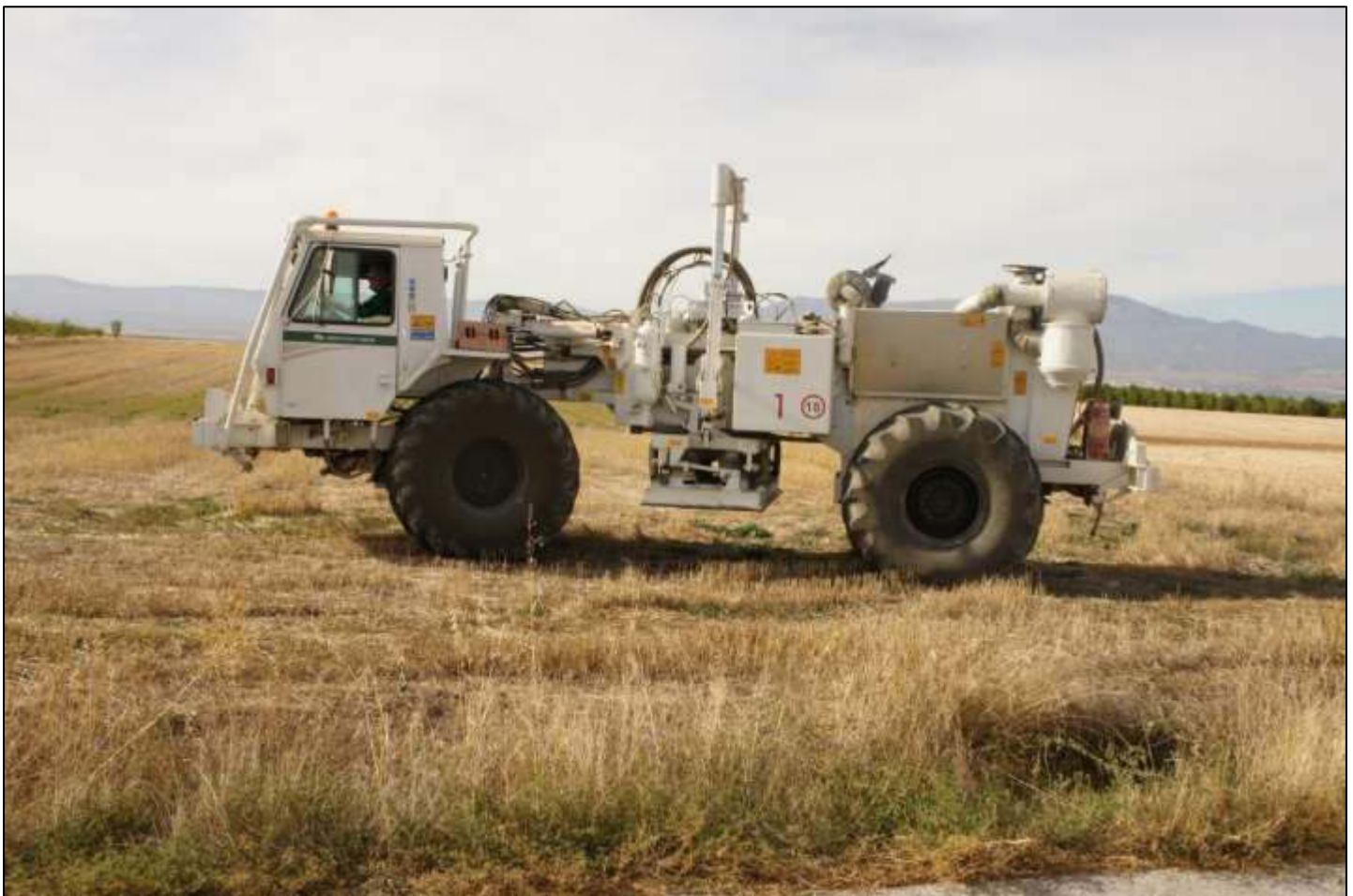
Plate 3.3: Vibroseis used as energy sources for onshore oil and gas exploration process (Source: REN, 2021).
