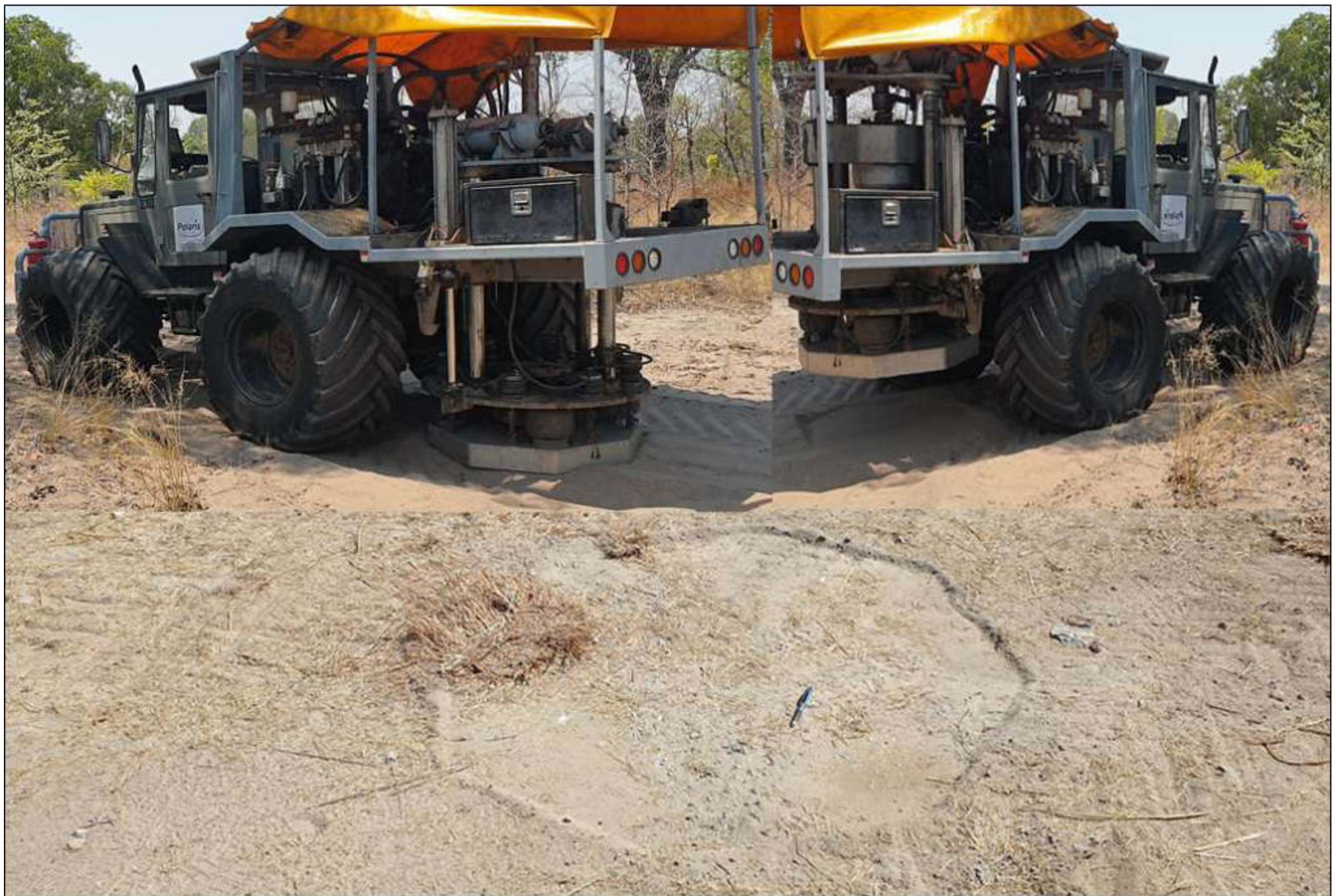
Plate 3.2: Ground footprint left by an Explorer 860 after data acquisition at each station along a given survey line.
