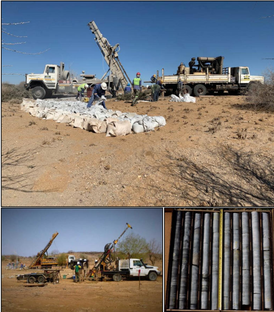
Fig. 13. RC and diamond drilling rigs at work also shown is drill core (activities are very localized with limited footprint).
