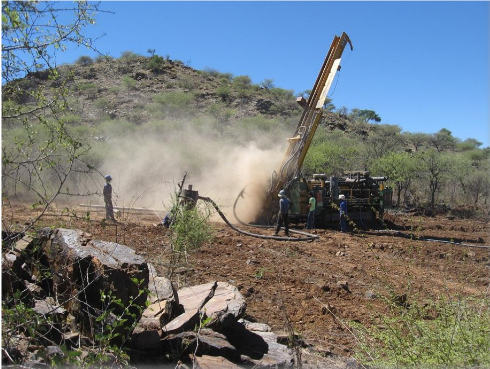
Crawler truck mounted R/C rig drilling an inclined hole
