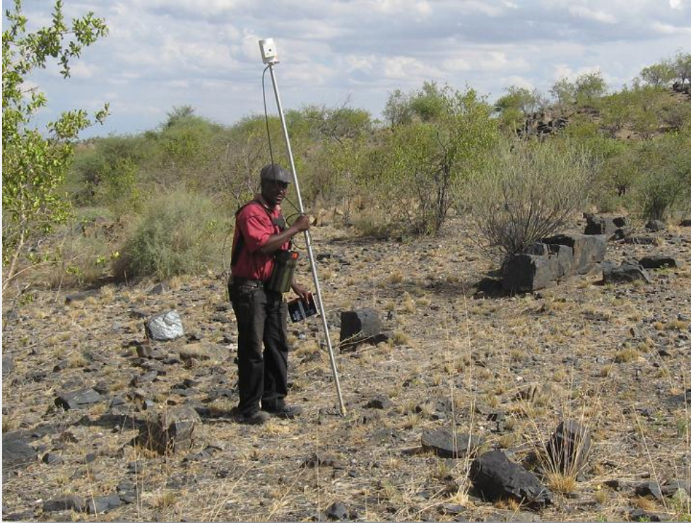
Fig. 2: Proton Precession Magnetometer Geometrics G-386 operated by a Geotechnician
