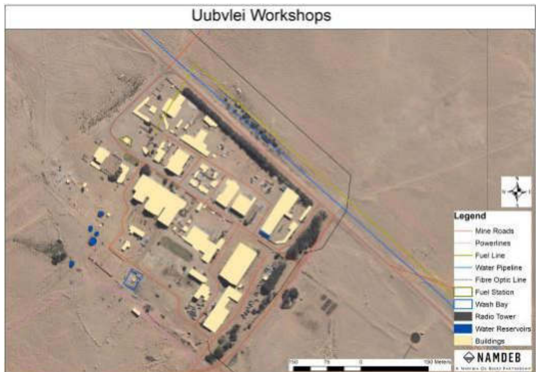
Figure 22. Infrastructure at Uubvlei workshops (map compiled by Namdeb, February 2021). Note that the path of the fuel line from the East-cliff road to the fuel station is only approximate, as it does not traverse a workshop.
