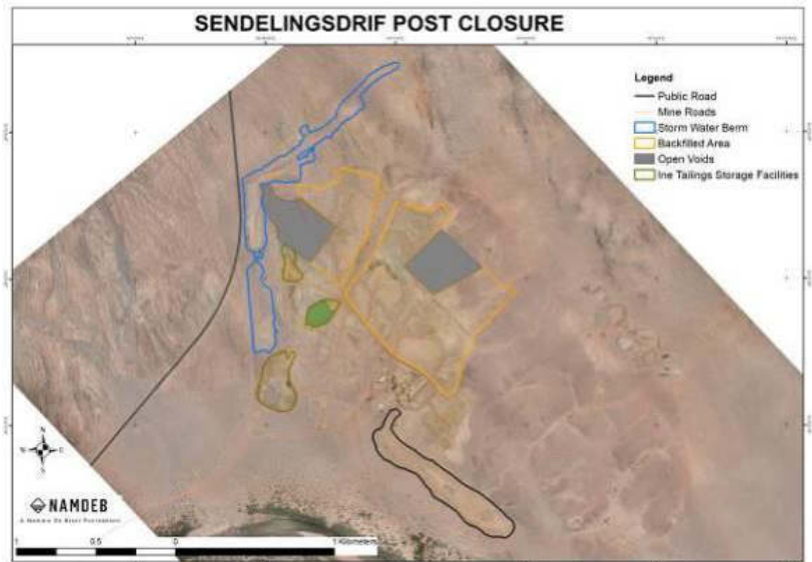
Figure 16. Features remaining at closure at Sendelingsdrif (the black outline is the tailings dump).
