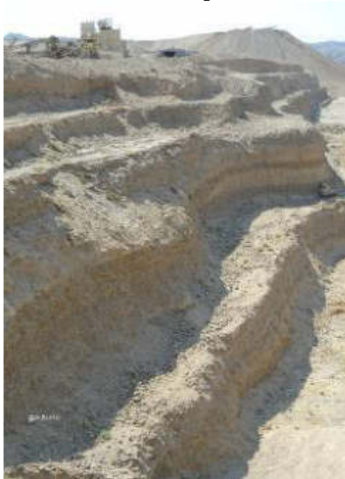
Figure 2: Benched slopes indicate where terraces have been excavated at Daberas (left). Mining operations at Sendelingsdrif (right) include backfilling the mine voids in the mine plan.
