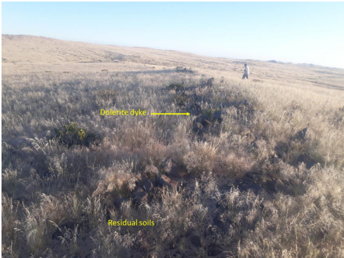
Figure 4-5: One of the locations where the targeted dolerite was observed, with residual soils from the weathering of surrounding rocks.
