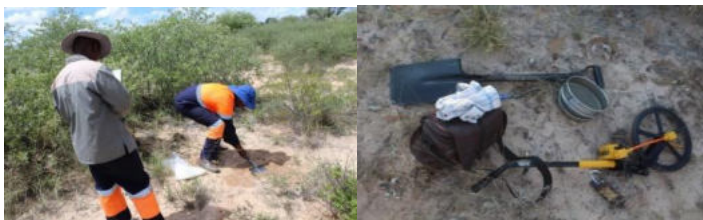
Figure 2-2: An example of soil sample collection and equipment (Resilient Environmental Solutions, 2019)
