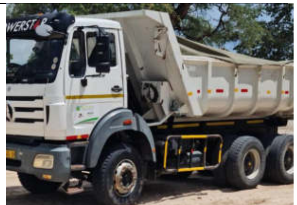
Sand mining delivery vehicle covered with canvas for dust control
