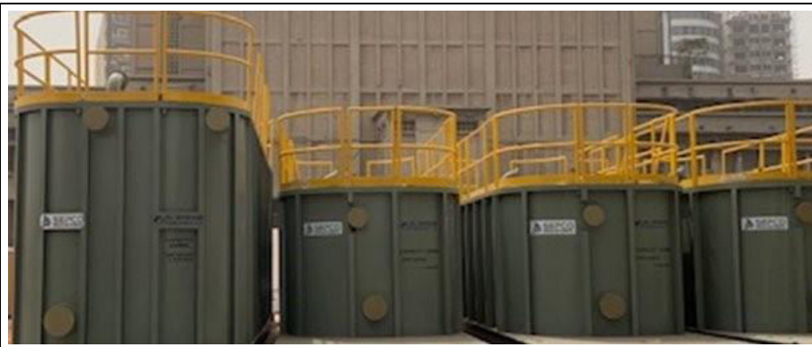
Figure ES-1-5: Example of fluid mixing tanks (Source: Halliburton, 2024)
