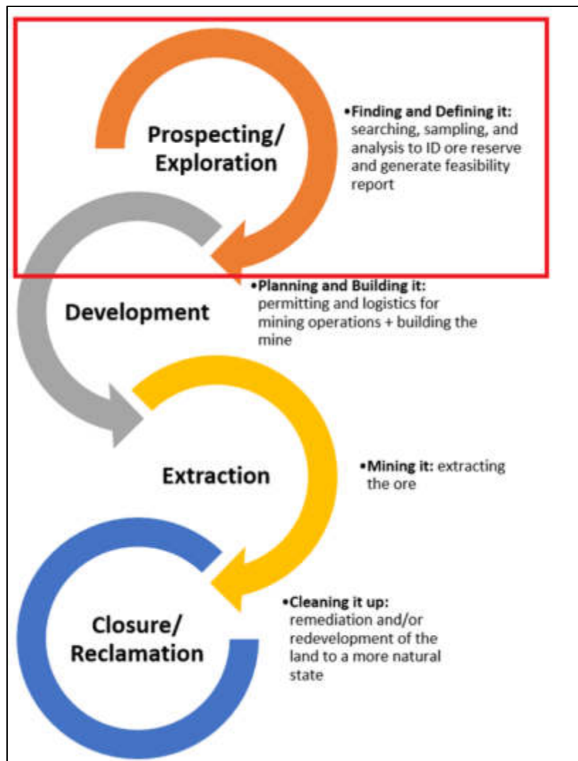
Figure 4: The Life Cycle of a Mine (The phase covered by this ESA study is highlighted in red, Excel Dynamic Solutions, 2021)
