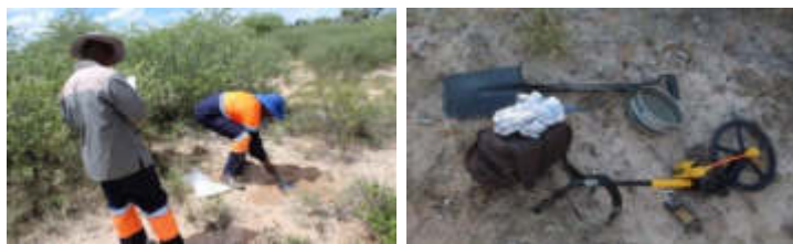
Figure 5: An example of soil sample collection and equipment (Resilient Environmental Solutions, 2019)
