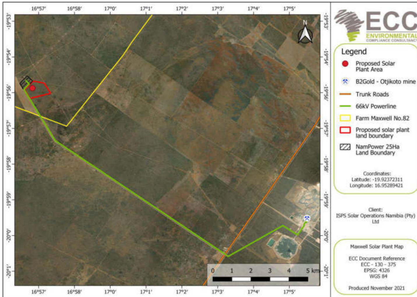
Figure 6 – Proposed solar PV power plant and powerline pathway to the Otjikoto mine
