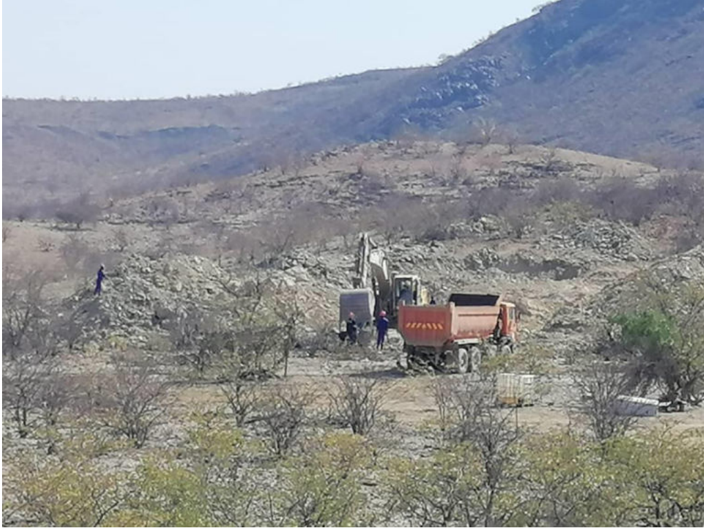
Figure 9: Copper ore will be explored for in trenches using both hand held tools and automated machines such as jack hammers and compressors (illustration purposes, HEEC, 2021).
