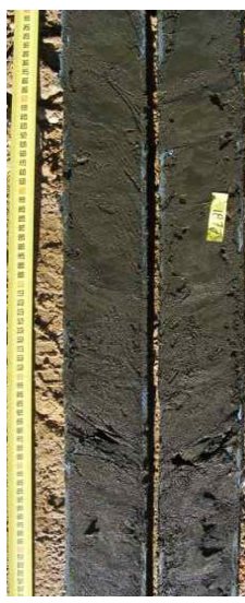
Figure 9 - Typical sedimentary sequence of the deposits with core 1877 showing both layers 1 and 2 of the deposit.
