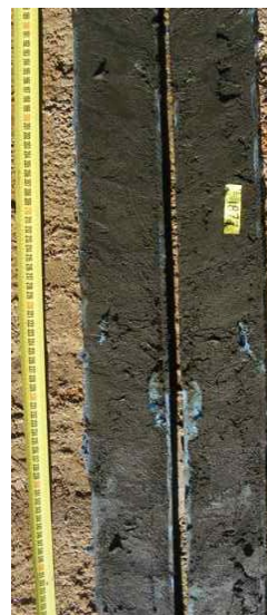
Figure 9 - Typical sedimentary sequence of the deposits with core 1877 showing both layers 1 and 2 of the deposit.
