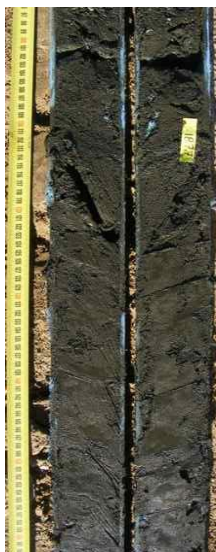
Figure 9 - Typical sedimentary sequence of the deposits with core 1877 showing both layers 1 and 2 of the deposit.
