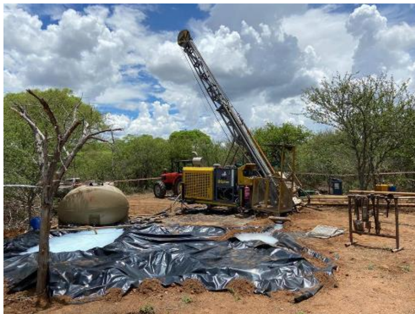
Figure 22 - Drill rig and sumps at site: NANAND000024
