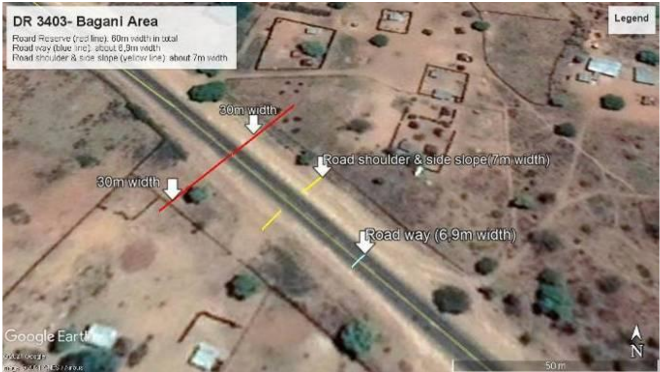
Figure 5: DR3403 Road reserve in already surfaced area, from Divundu to Bagani 13,5km in total of the 32.3km (Google earth, 2021)
