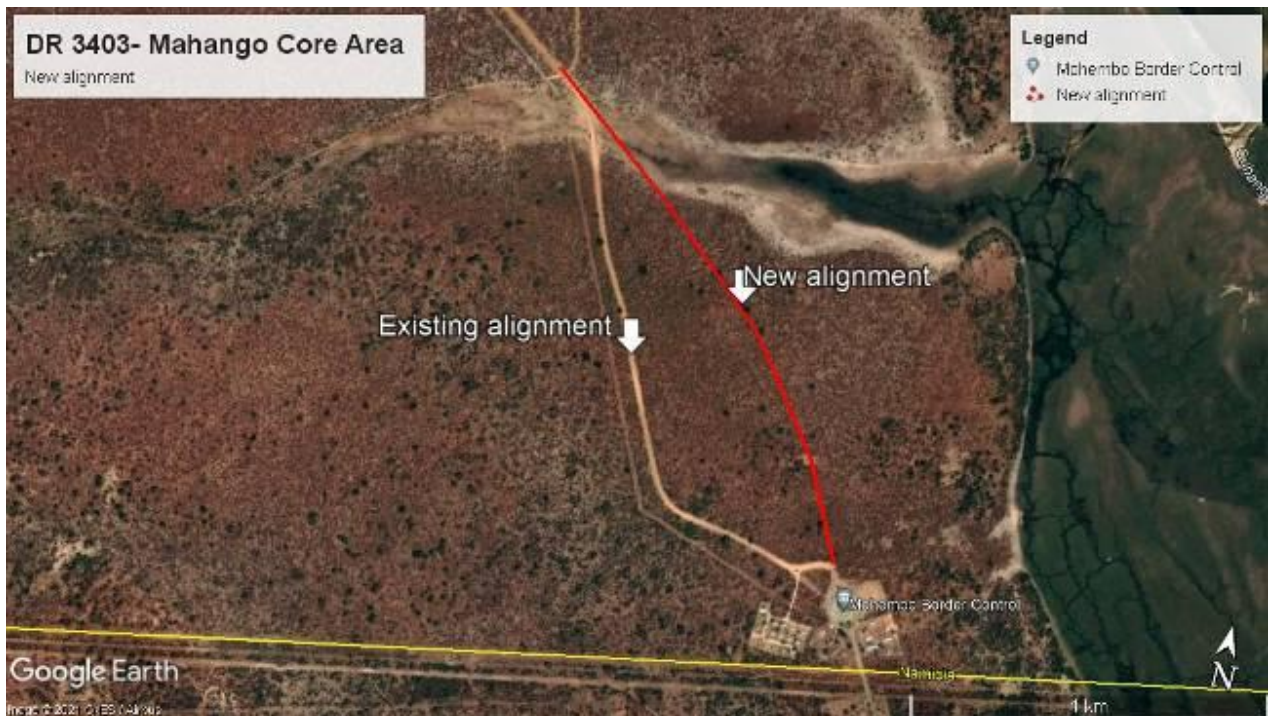
Figure 9: DR 3403 - New Alignment in Mahango Core Area (1,5km long)
