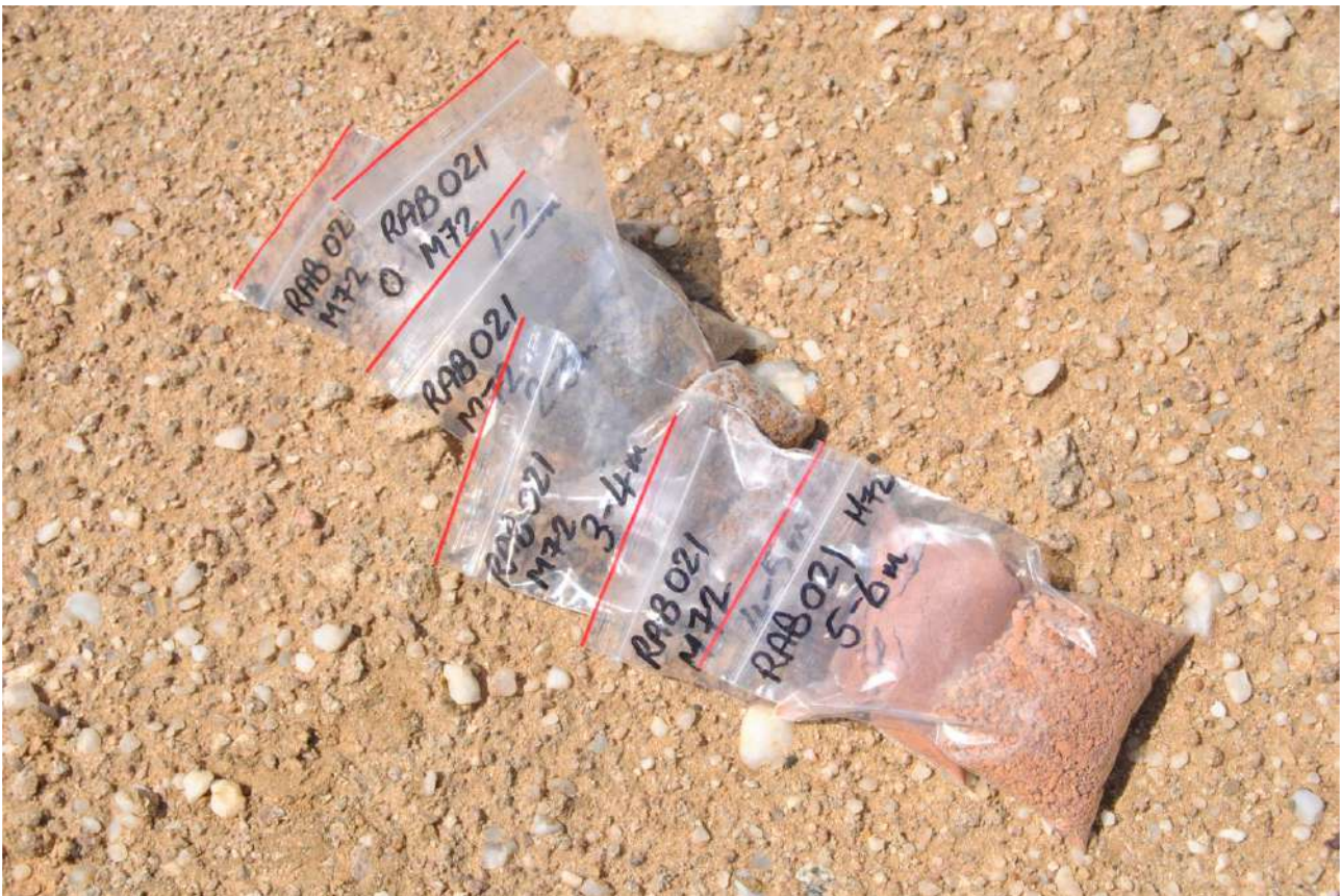
FIGURE 3 - SOIL SAMPLES BAGGED FOR LABORATORY TESTING
