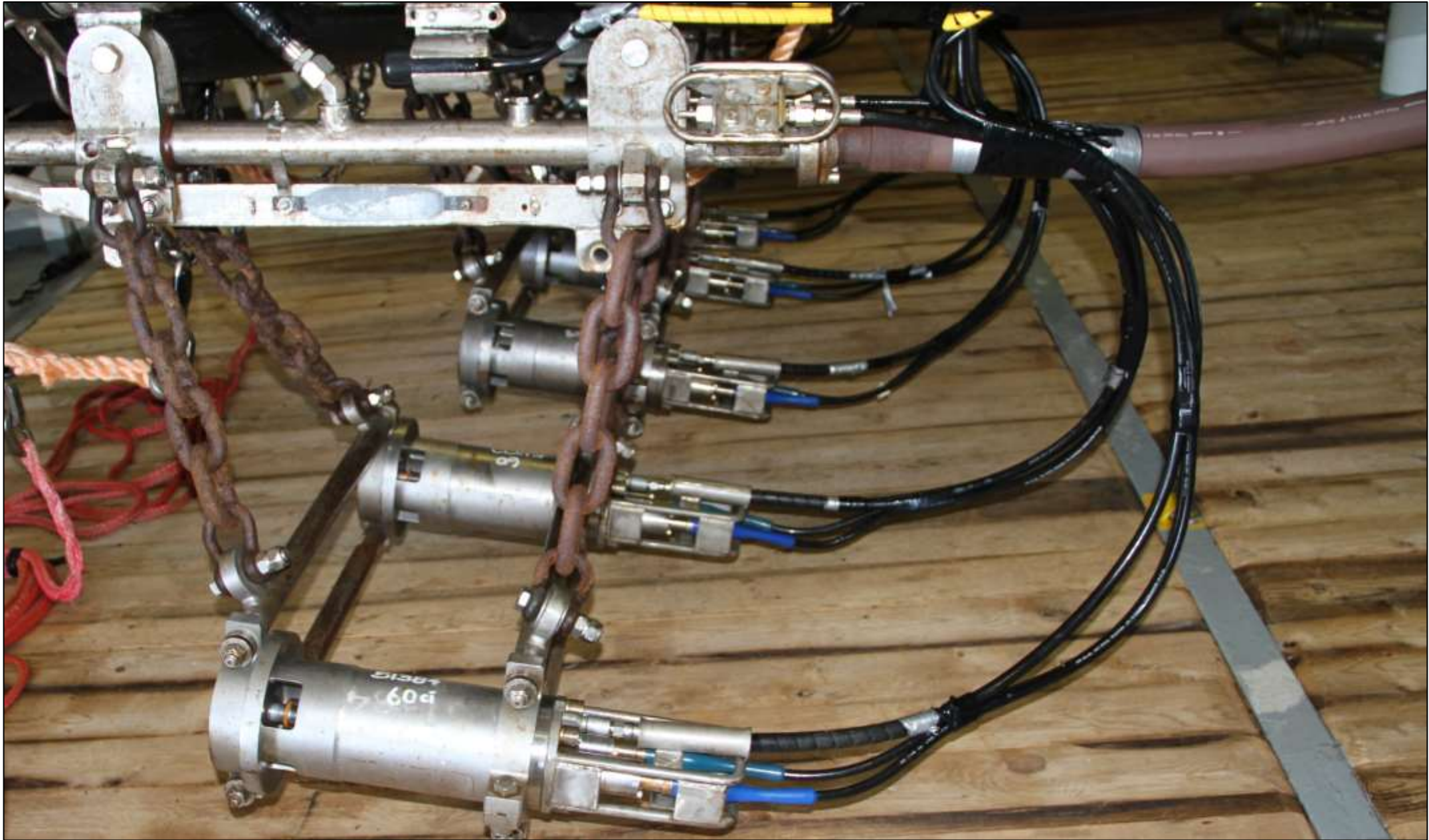
Plate 2.1: Example of the air guns used in marine seismic survey operations.
