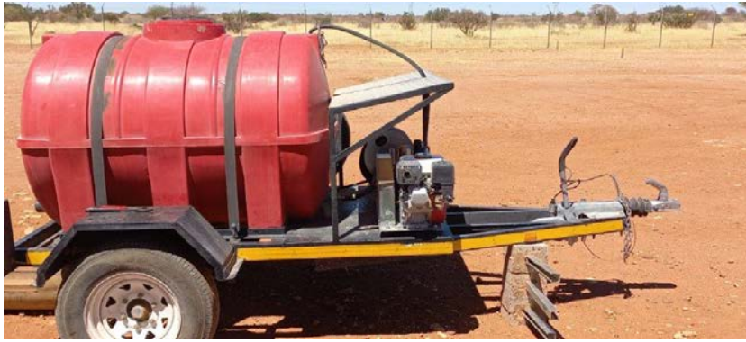
Photo 14 – View of firefighting trailer, operational and in good working condition.
