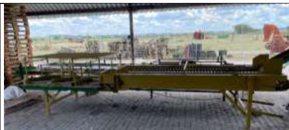
Photo 4-12 Potato washing and sorting equipment
