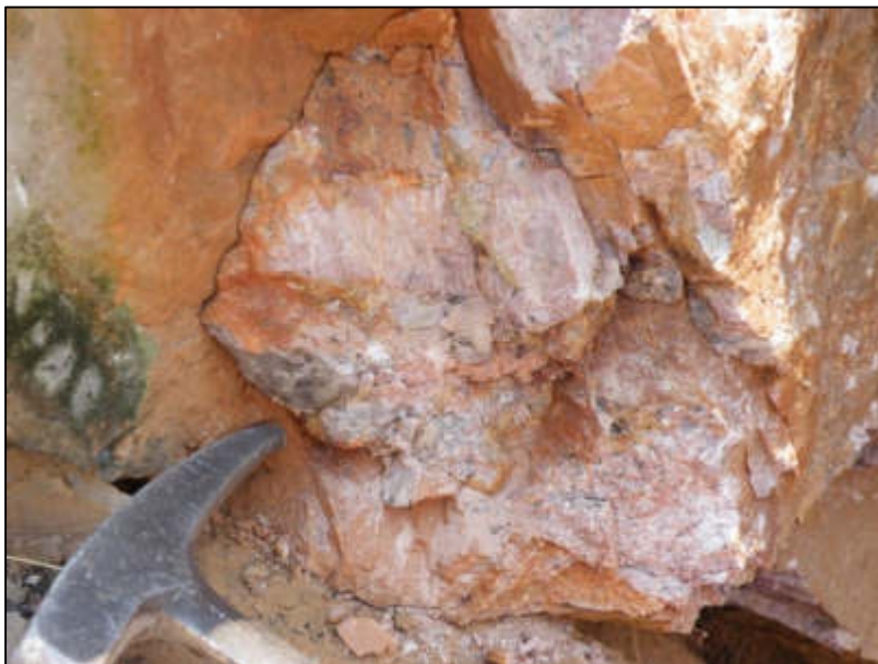
Fig. 14. Disseminated REE minerals in Q-Fsp vein.
