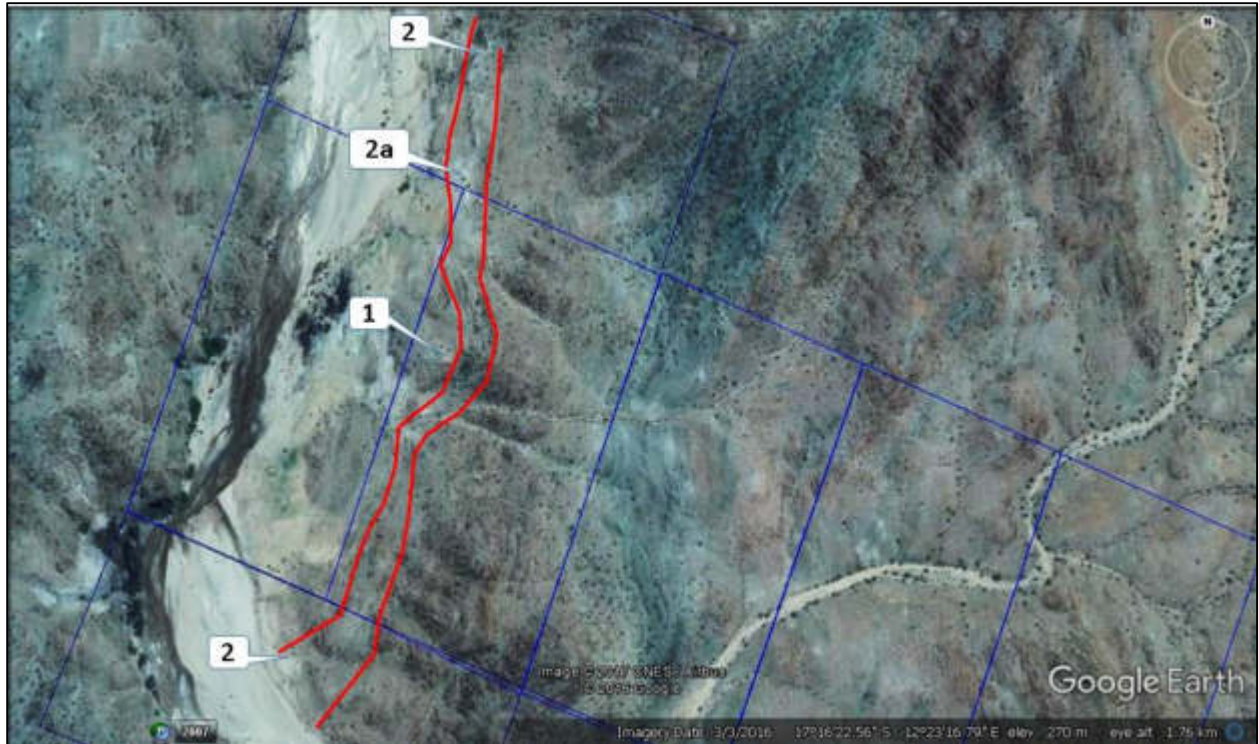
Fig.7. Shear zone on satellite image: 1- main REE deposit; 2 – outcrops of quartz-feldspathic veins with indication of REE mineralization (2a – visible REE mineralization).
