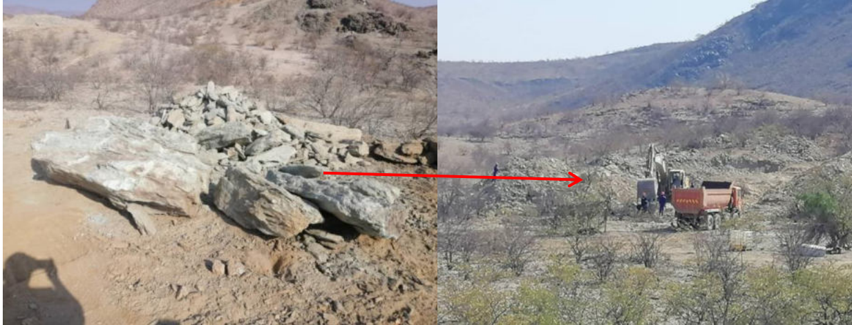
Figure 6: Copper ore will be extracted using both handheld tools and automated machines such as jack hammers and compressors, excavators and hauled with tipper trucks (HEEC, 2021).
