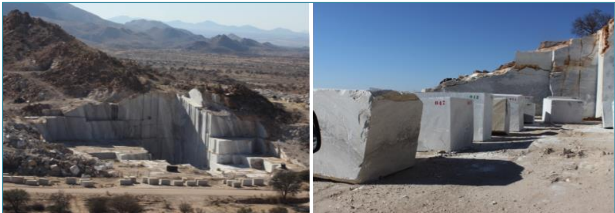
Fig 1: Shows general setup of a marble quarry where block are extracted and stored before being hauled to the harbour town for shipping (this is the least radioactive quarry activity).
