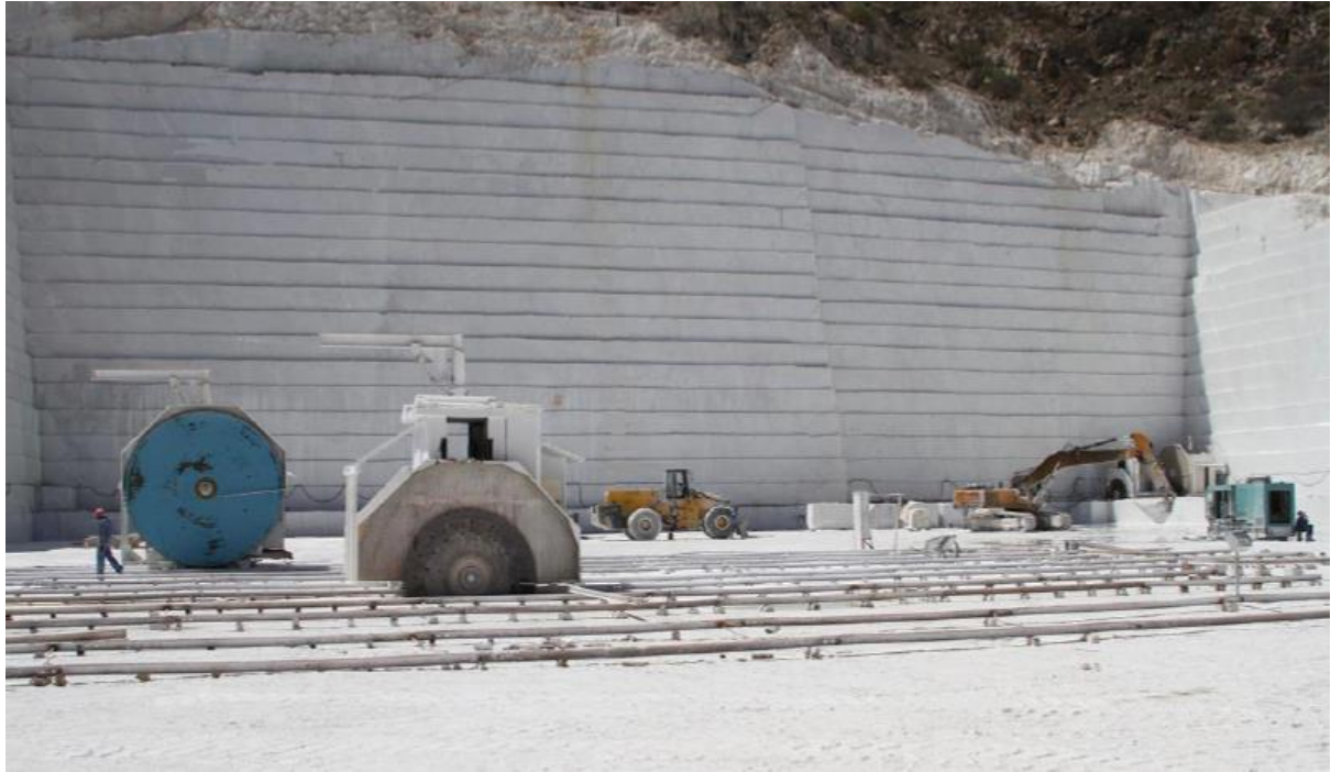
Figure 2-5. Typical quarrying and cutting operations in a dimension stone quarry
