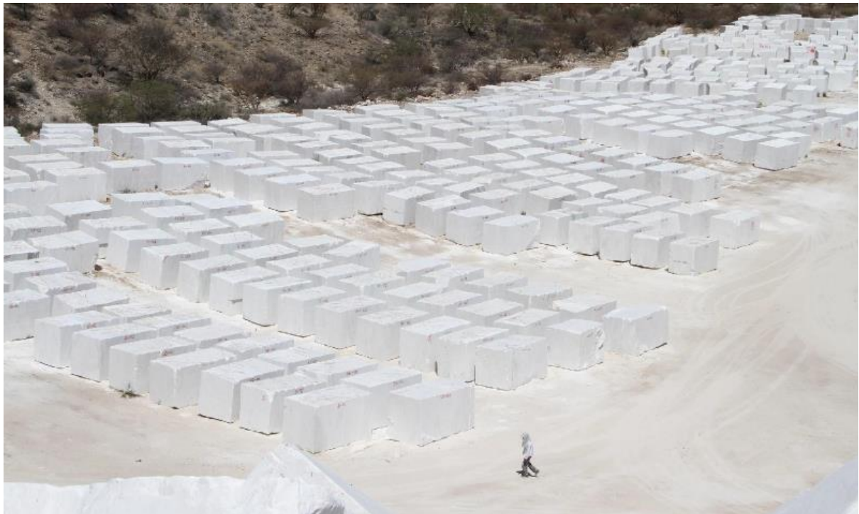
Figure 2-6. Typical on-site block sorting and stockpiling prior to transportation for further beneficiation
