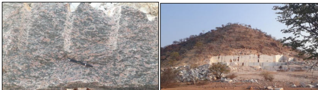
Figure 5.9. Red/ grey gneiss and white marble occurrence within the target area. The quarry exposures and extracted blocks are from previous quarrying in the area which ceased in 1997.
