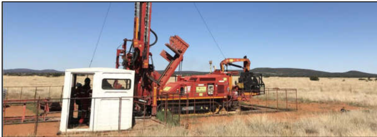
Figure 6: A typical example of a Down-The-Hole drill rig (OMAVI, 2020)
