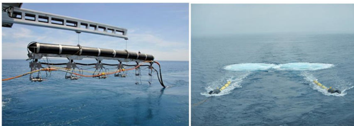
Figure 3-6: Example of a Seismic Source (Airgun Array)
