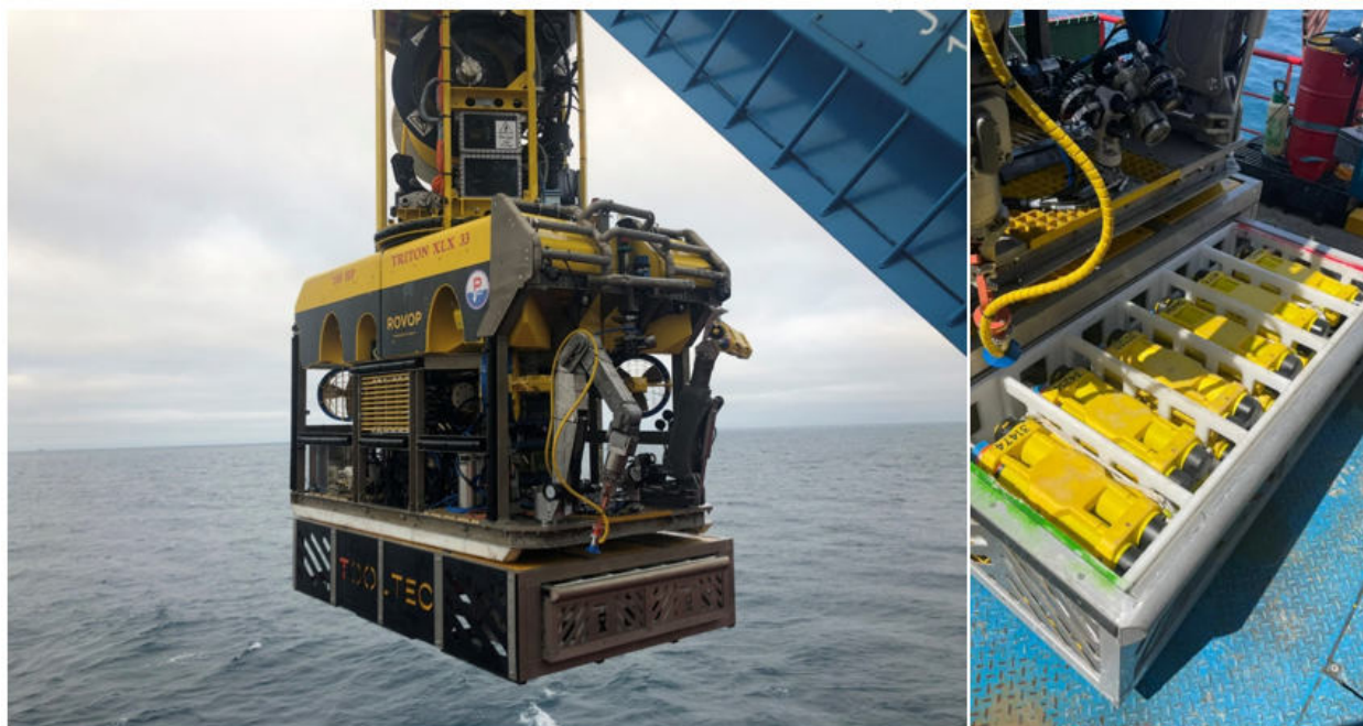
Figure 3-4: Example of a node deployment ROV Source: https://www.rovop.com/ocean-bottom-node-deployment-in-central-north-sea/
