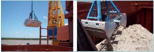
Figure 6: Illustration of the grab equipment used in the transfer of bulk mineral ore on a transhipment facility
