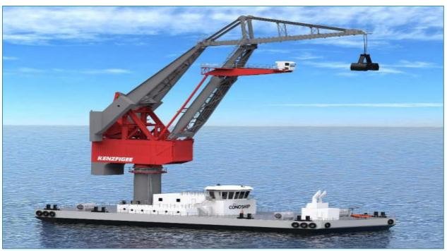
Figure 10: Shows a self-contained Floating Crane Transhipment Facility
