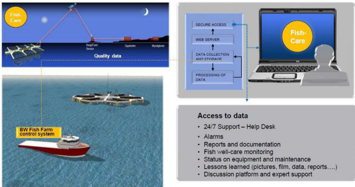
Figure 16: remote monitoring and logging technology system, designed by BW Offshore Farm, which will be installed (BW FishFarm, 2020).
