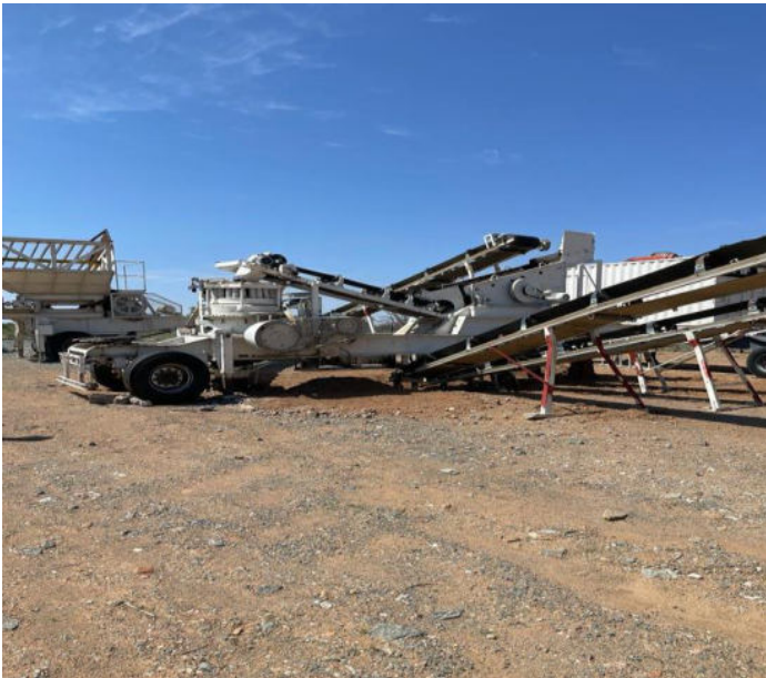
Figure 3: Illustration of a trailer mounted copper ore crusher
