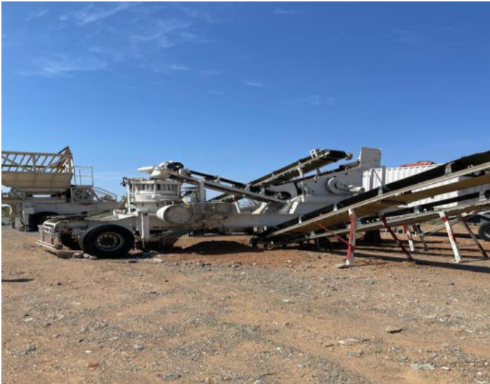
Figure 3. Illustration of a tailer mounted copper ore crusher.
