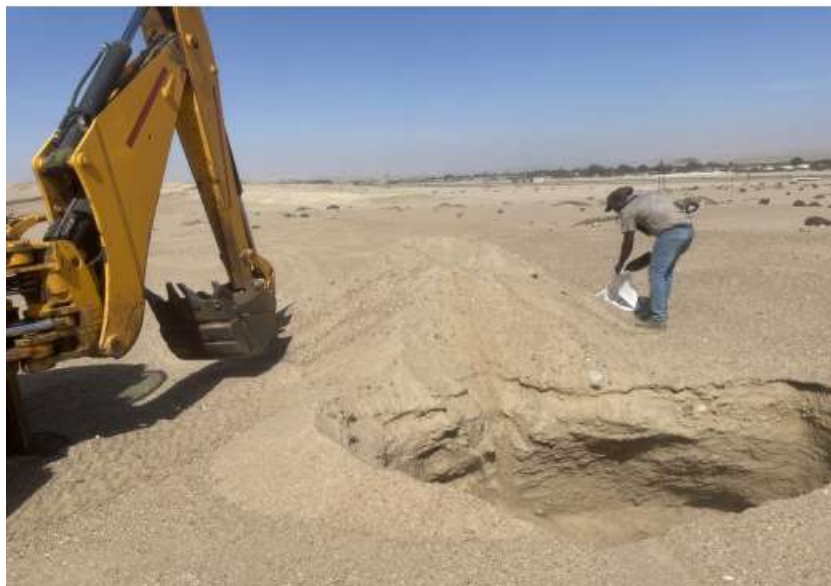
Picture 15 Alluvial coarse sand has been shown to be the dominant soil types across the site encountered in test pits at borrow pits.
