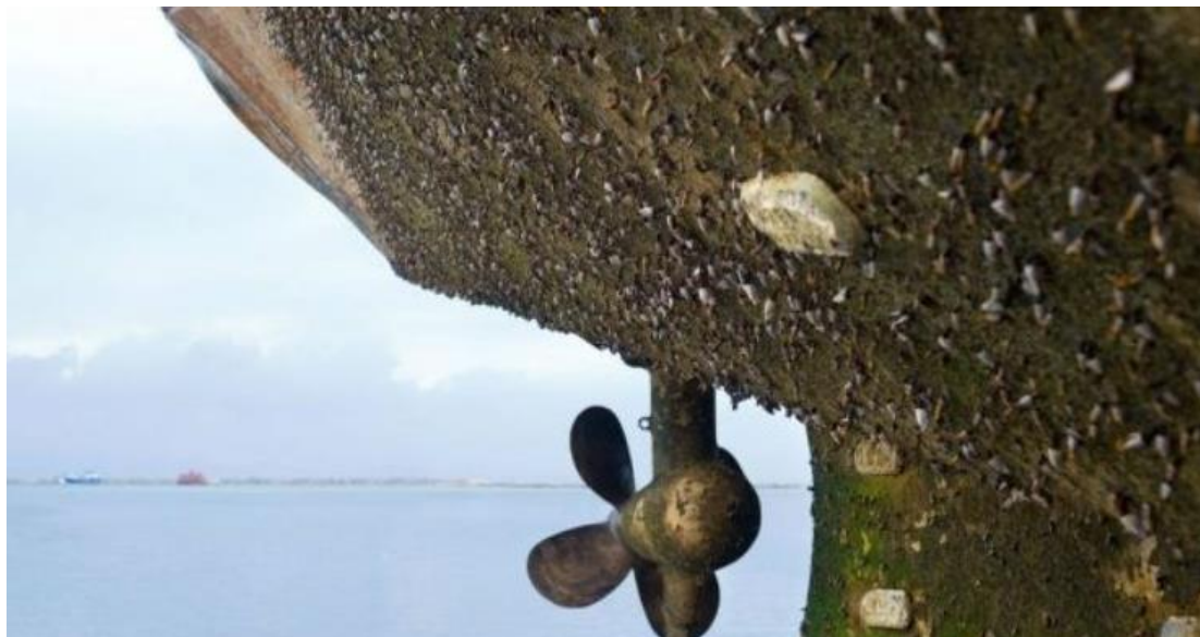
Figure 1: build-up of biofilms and fouling organisms increase vessel drag and fuel consumption (source: https://safety4sea.com/cm ).
