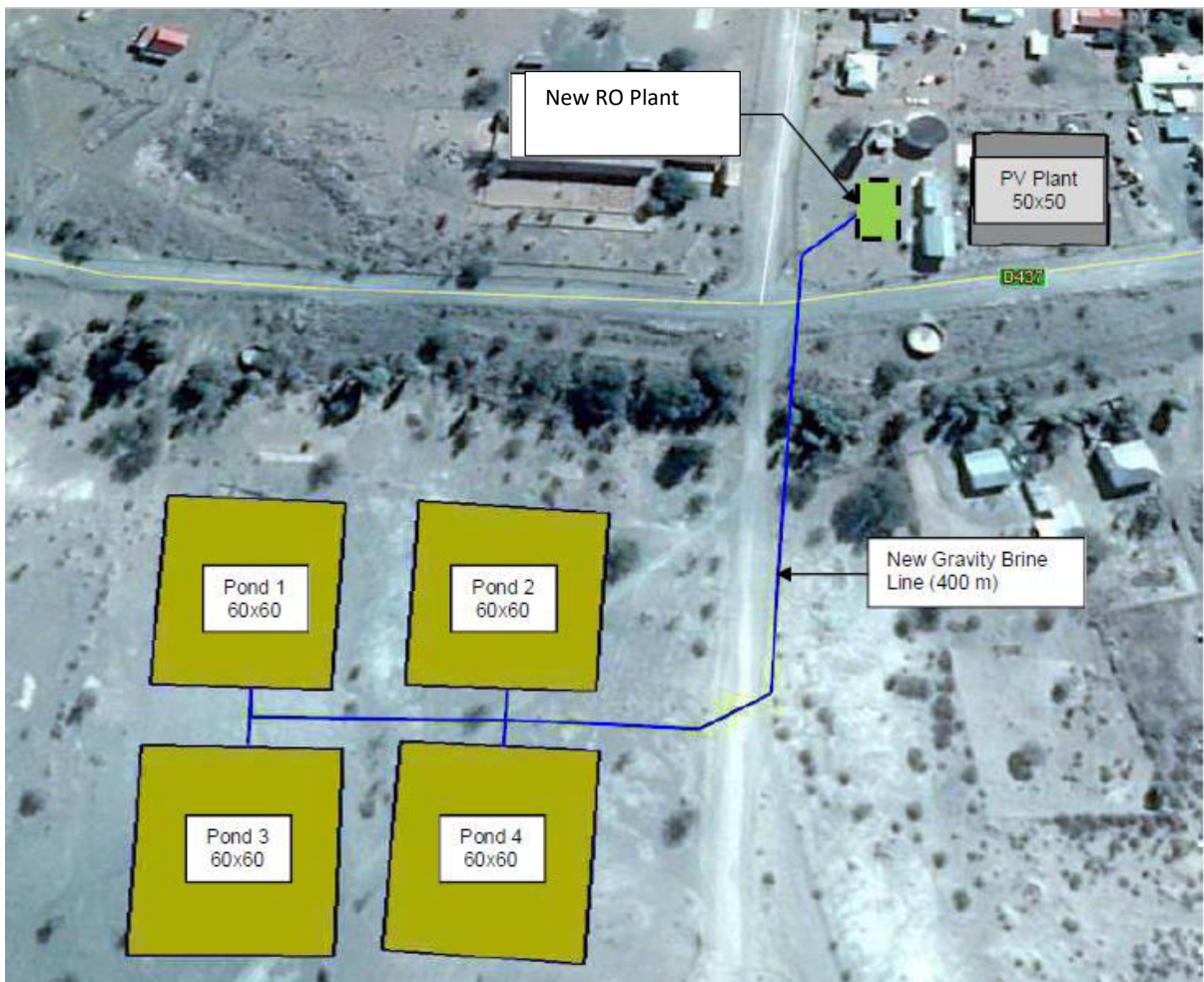
Figure 4: New Infrastructure Added to the Bethanie Plant
