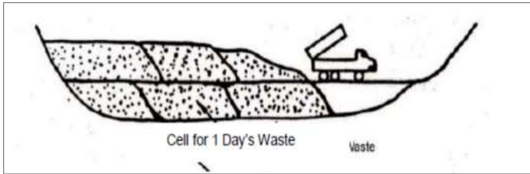
Figure 21 General waste cell landfilling approach
