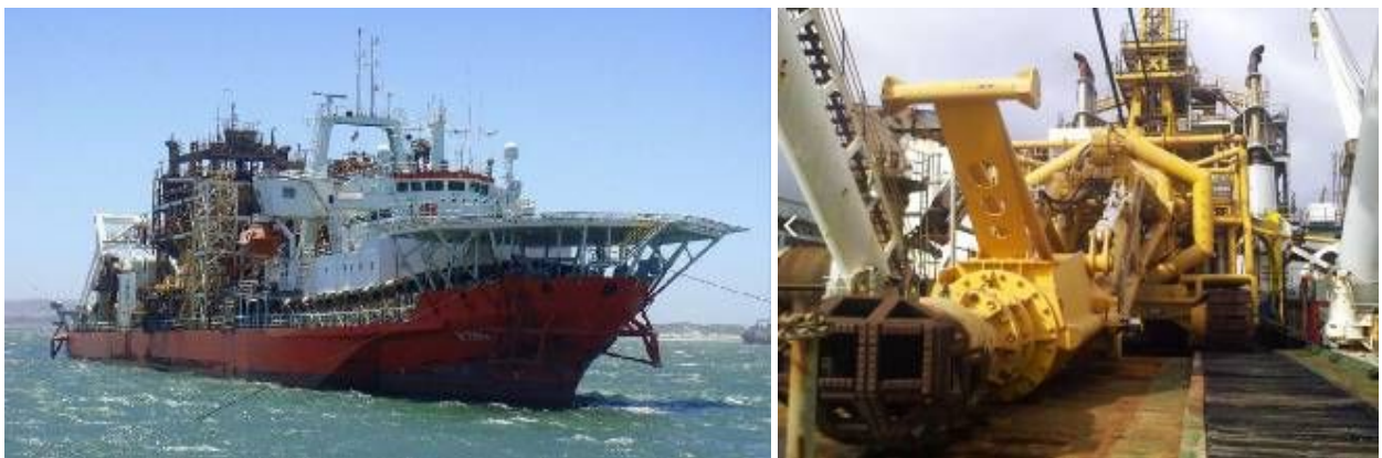
Figure 14. A typical mining vessel (left) and seabed crawler (right).
