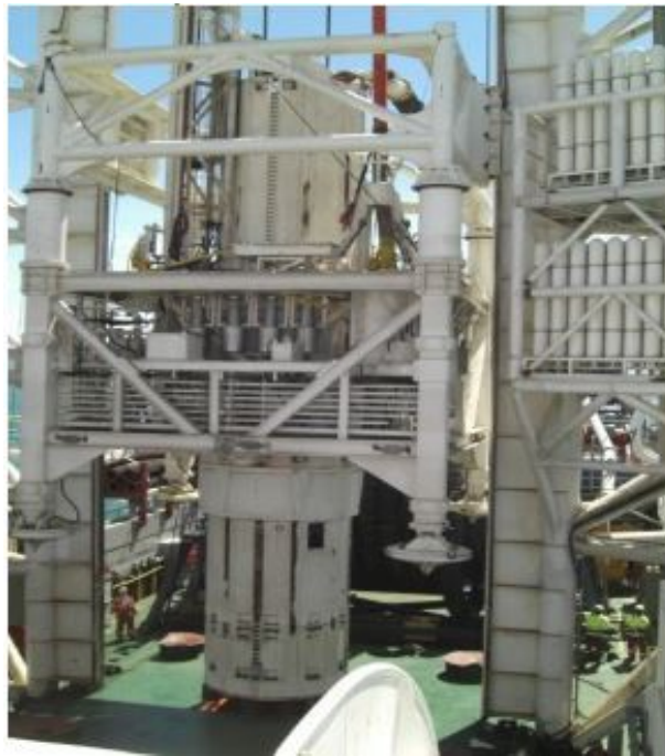
Figure 09. The 2.5m diameter drill bit within the drill frame structure.
