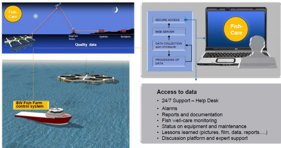
Figure 26: Remote monitoring and logging technology system, designed by BW Offshore Farm, which will be installed (BW FishFarm, 2020).
