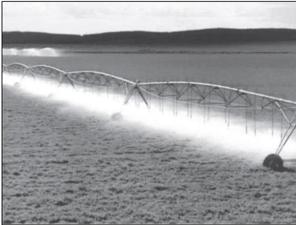
Figure 5: The Centre Pivot system overview (Phocaides, 2007)
