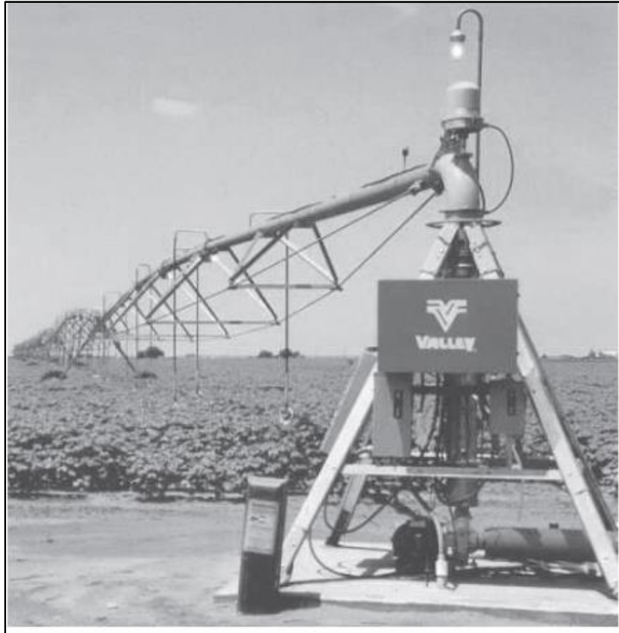
Figure 4: The Centre Pivot (Sprinkler) system (Phocaides, 2007)
