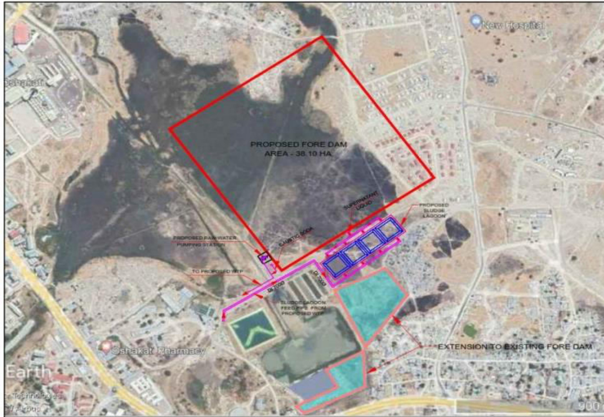
Figure 5-3 Design alternative 2 for raw water storage dam
