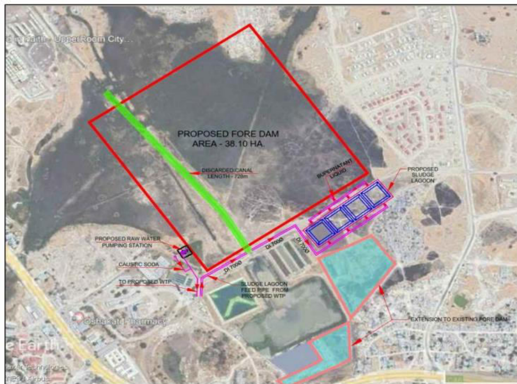
Figure 5-2 Design alternative 1 for raw water storage dam
