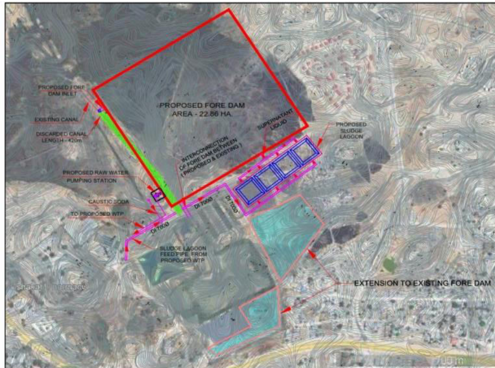
Figure 5-4 Design alternative 3 for raw water storage dam
