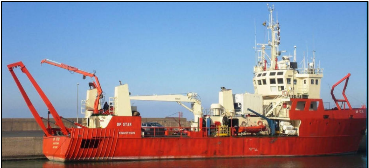
Figure 3.1: Dedicated geophysical survey vessel, mv DP Star, length overall 45 m.
