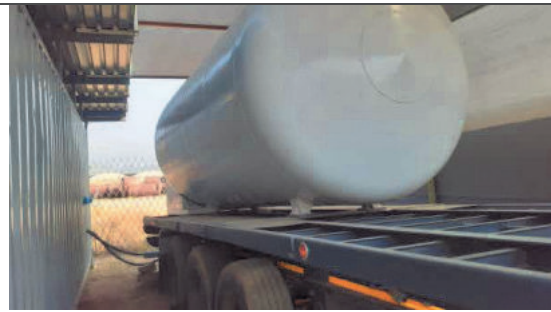
Photo 2-2 Mobile CO 2 tank
