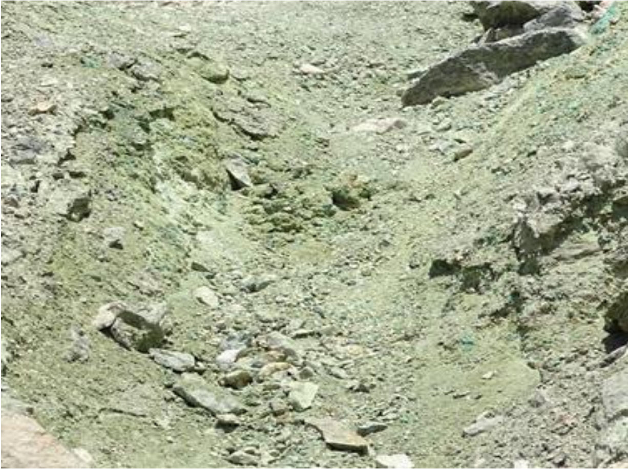
Photo 1 , Old Khan mine tailings showing copper green precipitation in the tailings.
