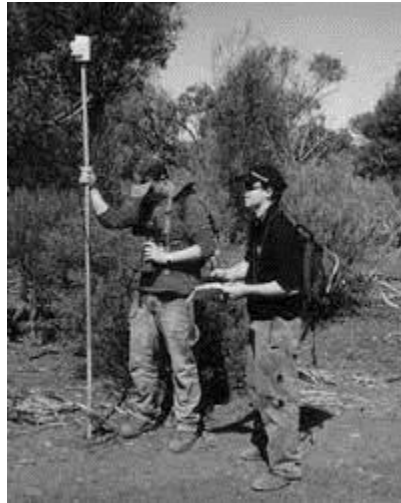
FIGURE 4- ILLUSTRATIVE IMAGE OF A GROUND-BASED GEOPHYSICAL SURVEY WITH MAGNETOMETER (Photo taken from: https://irsl.ss.ncu.edu.tw/media/course/CI/SIO_9.pdf )
